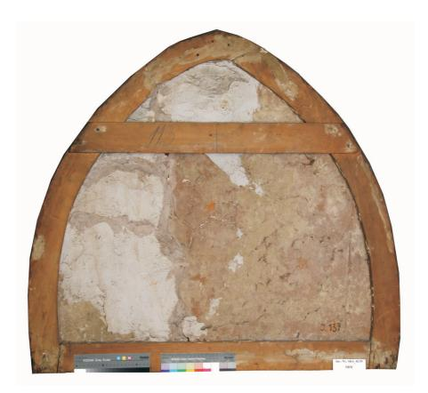
Fig. 3: Pre-state, back – ceramic relief with gypsum stabilization and supporting frame  $\hfill \odot$  C. Schneider.
