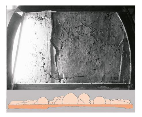
Fig. 10: Sidelight image of the backside after the removal of the mortar layers, schematic illustration (below) of a horizontal section trough the relief. The gaps between the lumps of clay, the vertical break parallel to the vertical offset due to the impression of the wooden board as well as the rectangular imprints of fabric panels around this edge are clearly visible. Photo: © C. Schneider.
