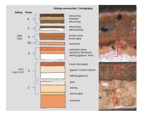
Fig. 7: Stratigraphy of painting layers. Photo: © C. Schneider.
