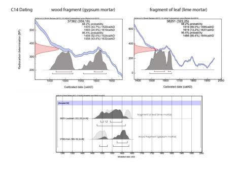
Fig. 9: Measurement diagrams C14 method. Individual measurements (top) and narrowing down the results using probability calculation (Bayesian model, bottom). Photo: © C. Schneider.
