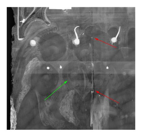
Fig. 10: Detail of x-radiograph of *Wedding at Cana/Dormition of the Virgin* showing the presence of wooden wedges in the joint (indicated with red arrows) and a strip of canvas added over the joint (indicated with a green arrow). Photo: René Gerritsen Kunst en Onderzoeksfotografie.
